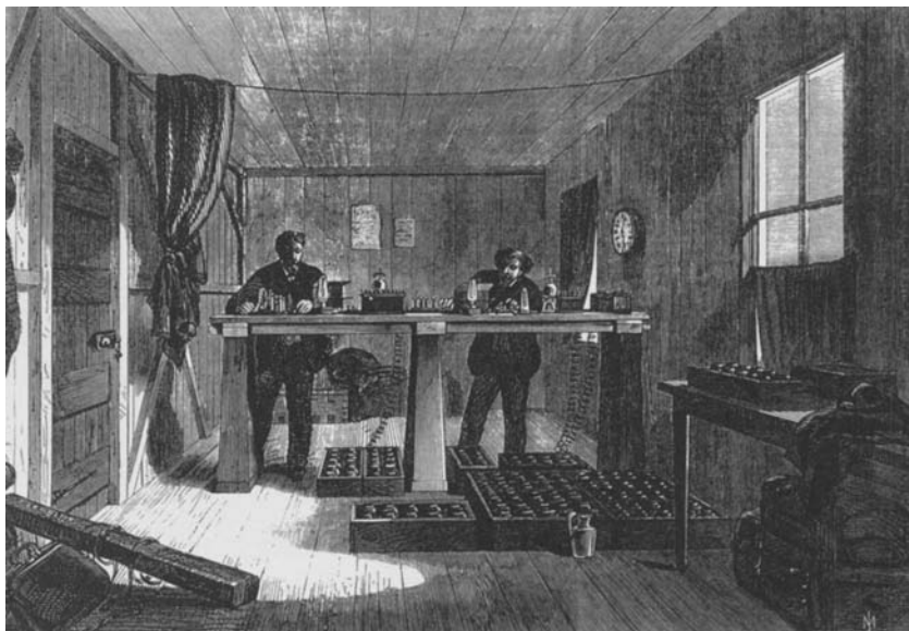
Figure 15.4 Signals from the Great Eastern being received in the instrument room at Valentia, Ireland, during the unsuccessful 1865 attempt to lay a cable across the Atlantic. Large chemical batteries are shown on the floor, and several of William Thomson's electrical instruments, including two of his sensitive mirror galvanometers, can be seen on the table. Similar instruments soon came into use in British physics laboratories. (From the Illustrated London News 47 [5 August 1865]: 117.)
